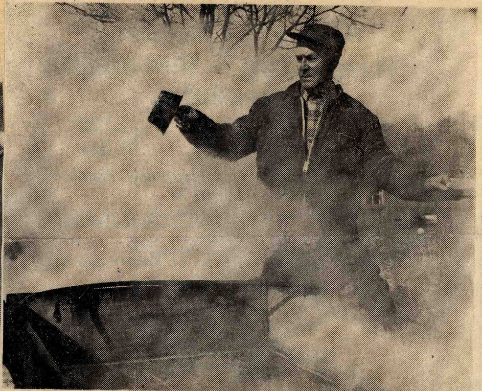
Mr. Page uses a small dipper to test whether the boiling sap is thick enough to take off as syrup.
