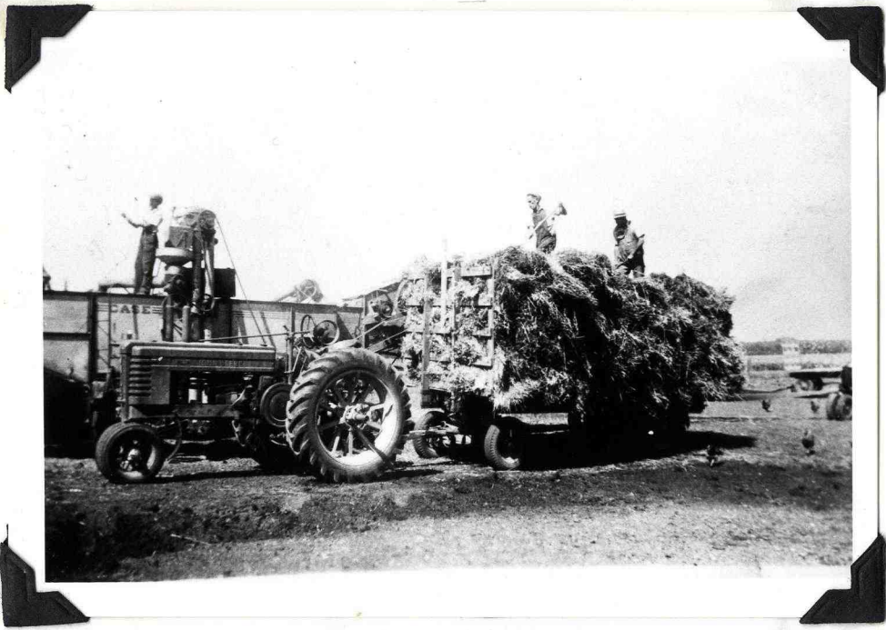
Threshing at W.E. "Bill" Walters' farm S \frac{1}{2} , Lot 13, Conc. 7, Yarmouth. Front-Bill's son, W. Robert "Bob" Walters (Front) Mait Muir-pitching sheaves (hired man); Charles "Toby" Ryckman, pitching sheaves of oats from wagon into threshing machine. Tractor is 1944 John Deere "B"
