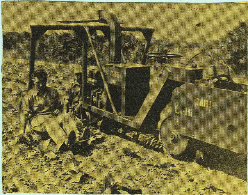
Picture of duster Showing seat attachment for picking suckers and sand leaves
