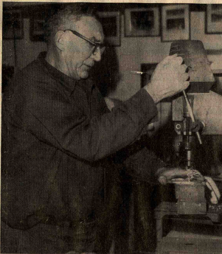
Ernie Murphy, a local blacksmith, uses a drill press to make cork holes in a horse shoe. Corks are small cleat-like pieces set at the front of a horse shoe.
